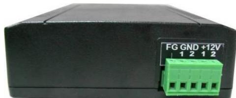
There are two separate 12V output connections Gnd (or V-) and +12V (or V+):
