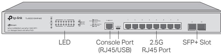
The front panel of TL-SG3428 V2.0 is shown as the following figure.
