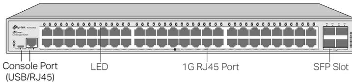
The front panel of TL-SG3452P is shown as the following figure.
