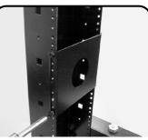
2 Secure the brackets to the rack using the #12x24 screws provided in the rear channel mounting holes only. Note: Four screws are provided for each bracket - two for the front and two for the rear.
