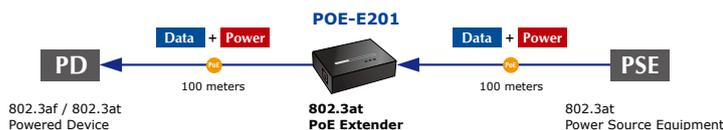
Providing high power PoE and Gigabit Ethernet data extension ability, the POE-E201 is an ideal solution for service providers, campuses and public areas networking applications which require PoE deployment of wireless access points, IP-Based surveillance or IP phones in any places. It enables you to centrally manage the power easily, efficiently and cost effectively.
