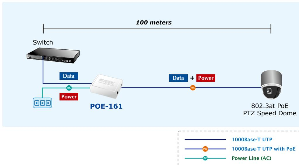
*The IEEE 802.3at Injector and Splitter Installation*
