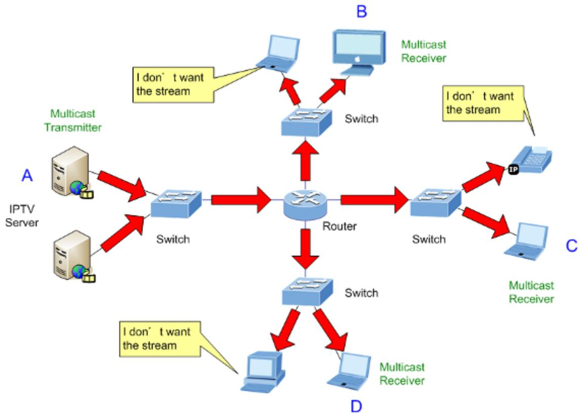
Figure 4-7-4: Multicast Flooding
