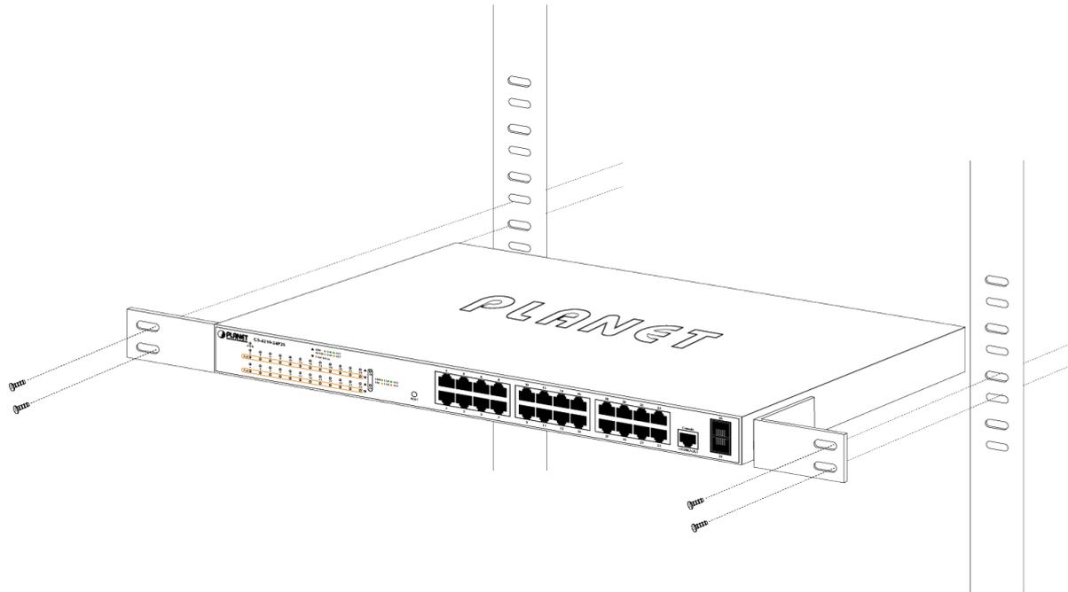
Figure 2-1-11: Mounting Managed Switch in a Rack
