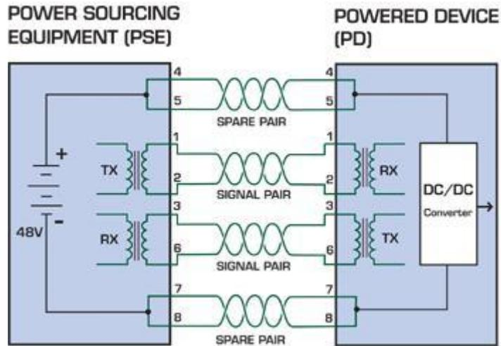
Figure 8-1: Power Supplied over the Spare Pins
