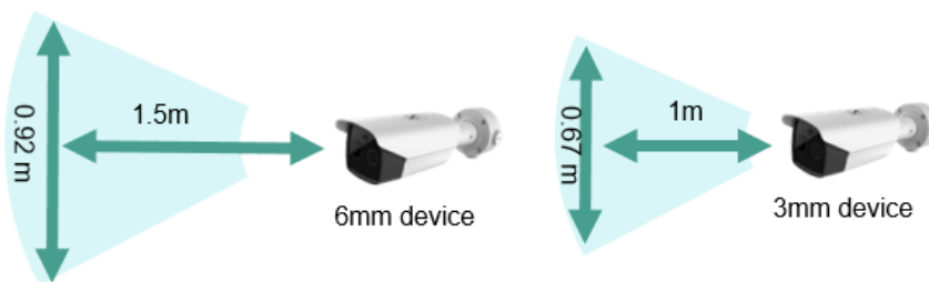
Thermographic fever screening scheme cover range
