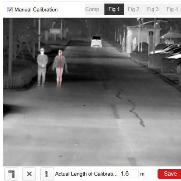
Figure 9-19 Manual Calibration (1)
