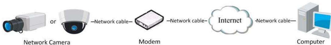
Figure 2-12 Accessing the Camera with Dynamic IP
