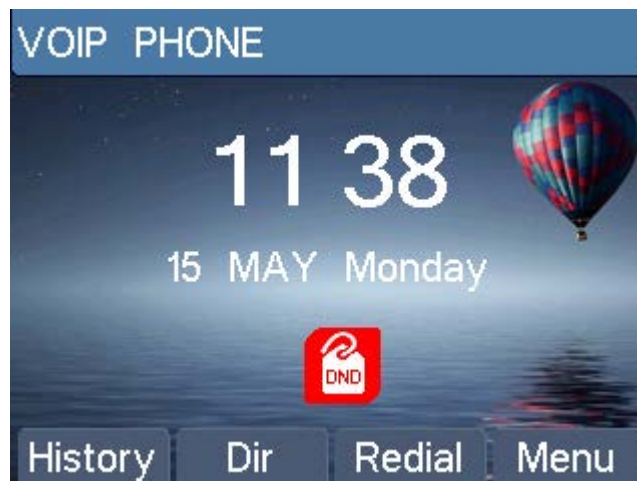
Figure 56 - DND Enabled on All Lines
