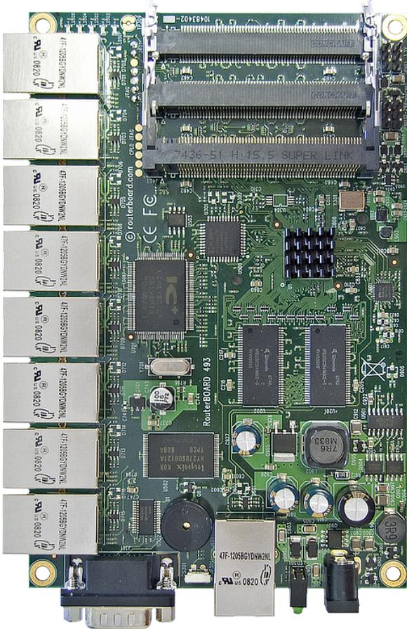
The RB493AH has nine ethernet ports and three miniPCI slots, it also has a switch chip, so the ethernet ports 2-9 can be grouped together to make it act as a switch.
